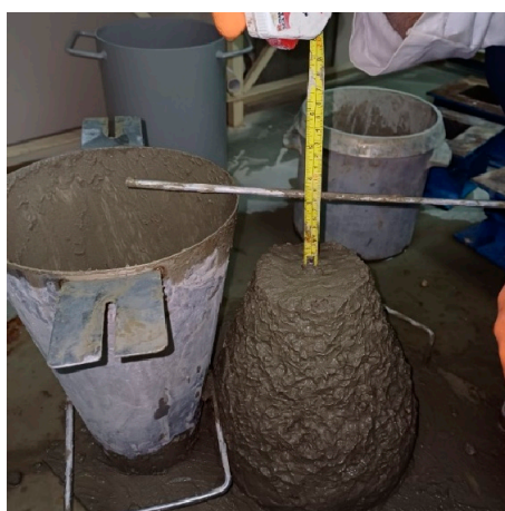
Figure 4. Workability or slump value measurement.
