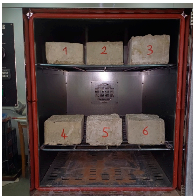
Figure 14. The rectangular prisms or half-cube specimens in the oven.
