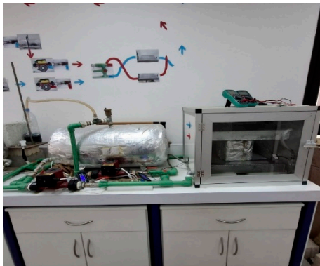
Figure 5. The flux metric method thermal testing setup.
