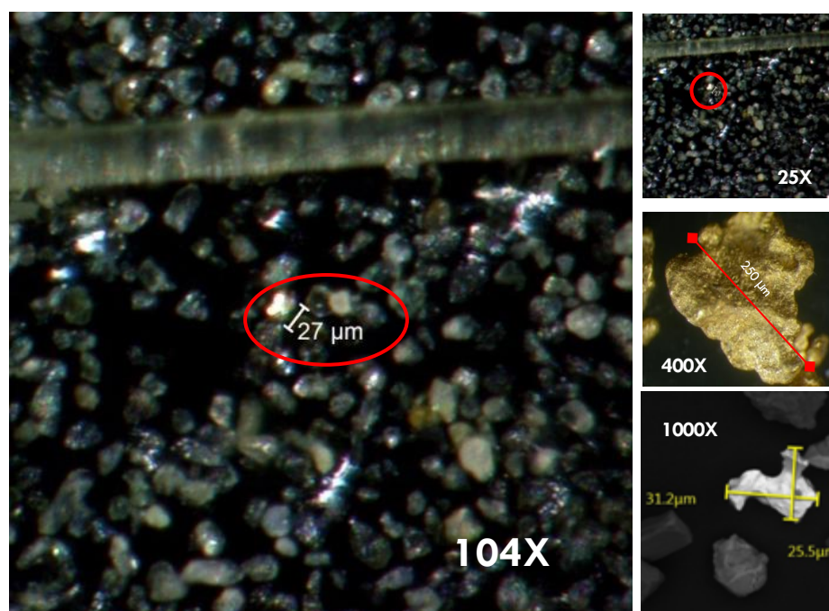
Figure 4. Examples of gold grains as seen at various magnifications with different types of microscope.
