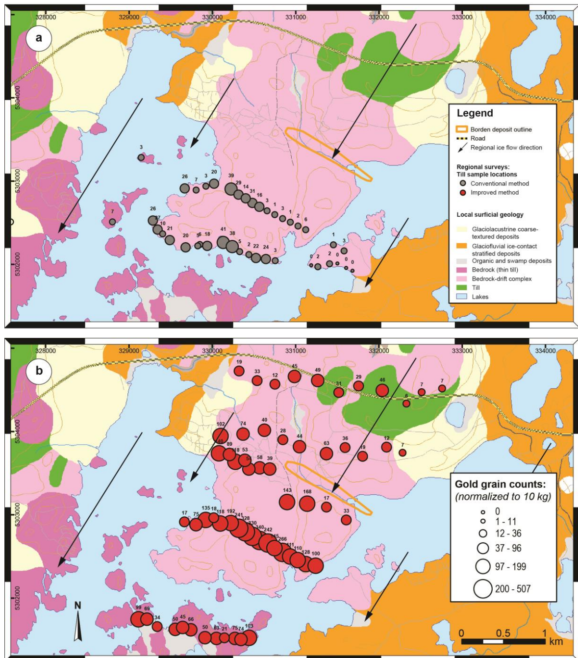
Figure 8. Map of the local area surrounding the Borden gold deposit showing surficial geology and locations of till samples (orientation surveys) processed with the conventional method (a) and the improved method (b). Note the number of samples for the conventional n = 40 and for the improved method n = 61 . The bubble diameter refers to the gold grain count normalized to a 10 kg sample. On the main profile down-ice of the deposit, samples for the improved method were collected in the same location within GPS accuracy from the previous conventional survey and can be considered as paired samples.
