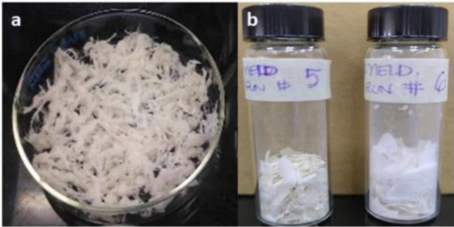
Figure 5. Cotton linters converted from a) cellulose to b) cellulose whiskers.
