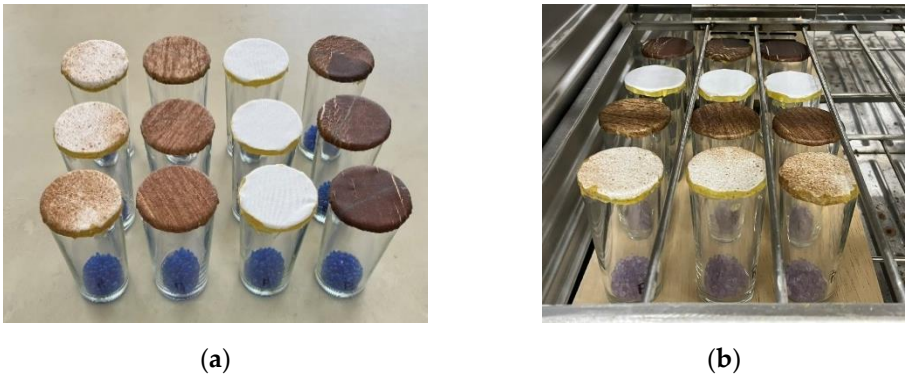
Figure 8. (a) Overview of the samples in the sealed test vessels before water adsorption, (b) Overview of the samples in the sealed test vessels after water adsorption and climate chamber conditions used in the determination of the water vapor transmission rate.
