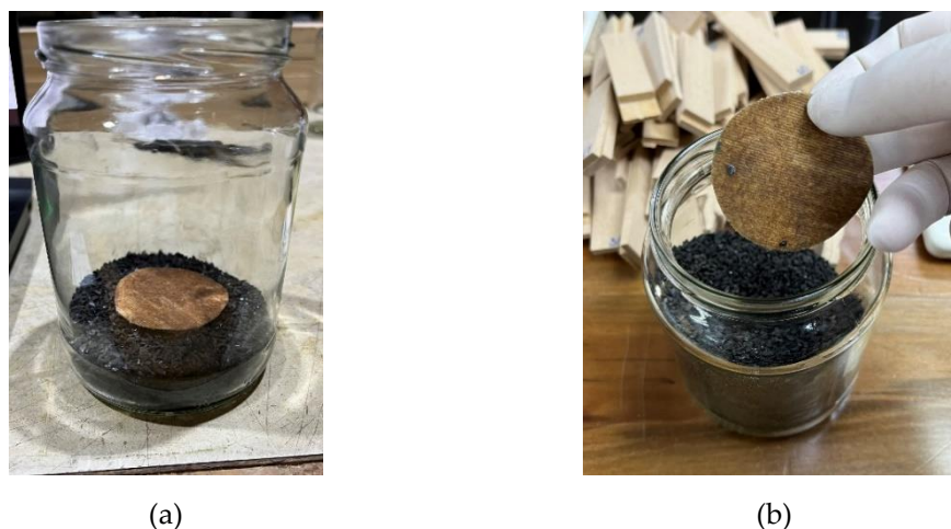
Figure 10. (a) Visualization of the textile samples in the test vessel containing the activated carbon: a) during the trial, (b) Visualization of the textile samples in the test vessel containing the activated carbon at the end of the trial.
