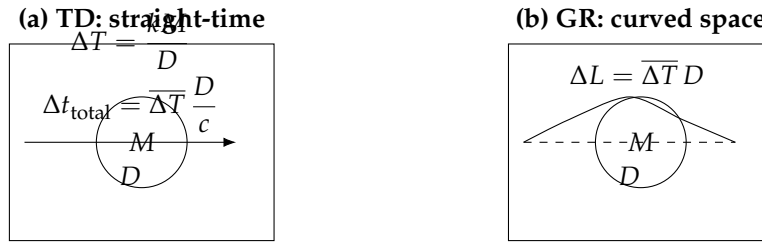
Figure 1. Two rulers describing the same physics. (a) TD: mass creates a local slow-time fraction \Delta T along a straight diameter D ; the integrated delay is \Delta t_{\text{total}} = \overline{\Delta T} D/c . (b) GR: the same effect appears as an added curve length \Delta L = \overline{\Delta T} D . With k = 4G/c^2 one gets \Delta L_{\text{rad}} = r_s and \Delta L_{\text{diam}} = 2r_s .
