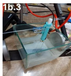
Figure 1. Diagrams of the CBD-HVEF-A (a) and CBD-HVEF-B (b) arrangements for electric field-assisted bath deposition. Electric field is induced by: (a) a voltage between two parallel plates placed on opposite outer walls of the glass vessel and (b) a voltage between the conductive substrate (ITO glass) immersed in the precursor solution and a metallic plate placed on the outer wall of the glass vessel. (c) Images of both systems.
