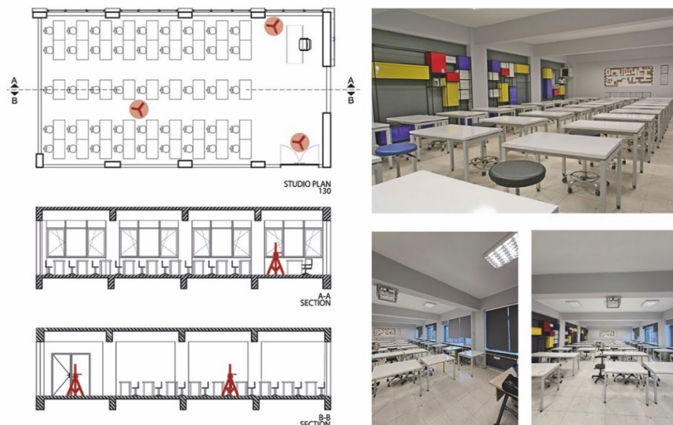
Figure 4. Measurement points and studio plan.
