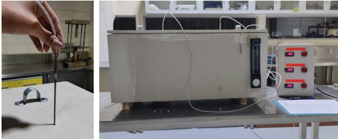
Figure 12. Data collection with thermocouple at intervals of 1, 30 and 60 minutes.
