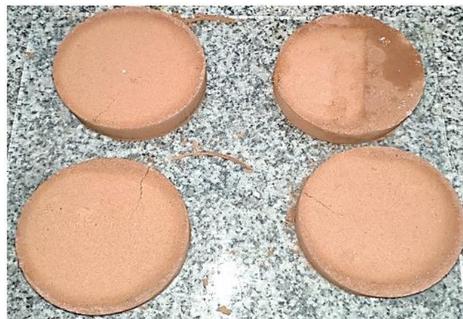
Figure 8. Cracks generated due to excessive curing temperature.
