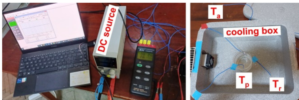
Figure 3. Experimental rig for the refrigeration system testing with water cooling load.
