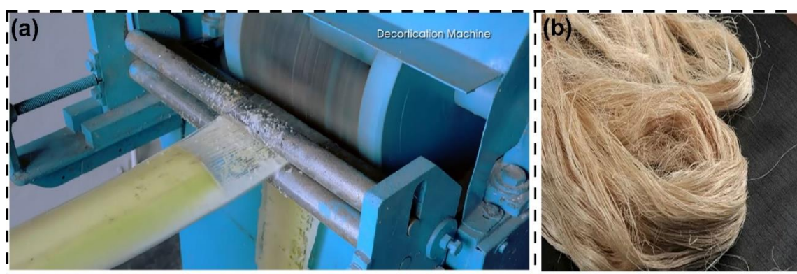
Figure 6. (a) Machine for mechanical extraction of banana fiber, (b) extracted banana fiber.
