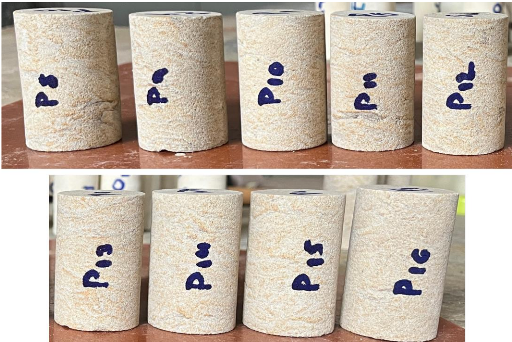
Figure 3. Experimental samples of sandstone with height h = 55 mm.
