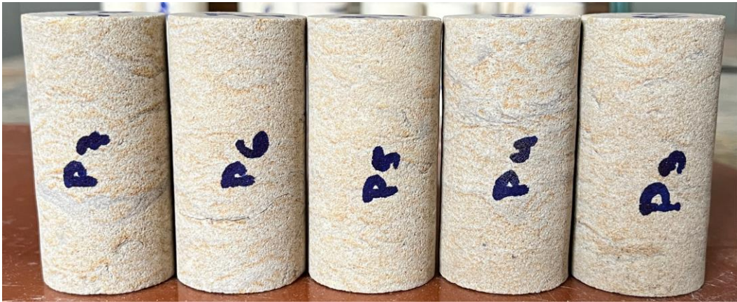
Figure 4. Experimental samples of sandstone with height h = 70 mm.
