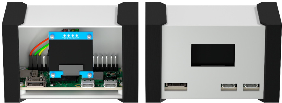
Figure 4. Renders of the control subsystem that utilised the Raspberry Pi Zero 2 W. The models for the Zero 2 W, and the display were sourced from [19] and [20], respectively.
