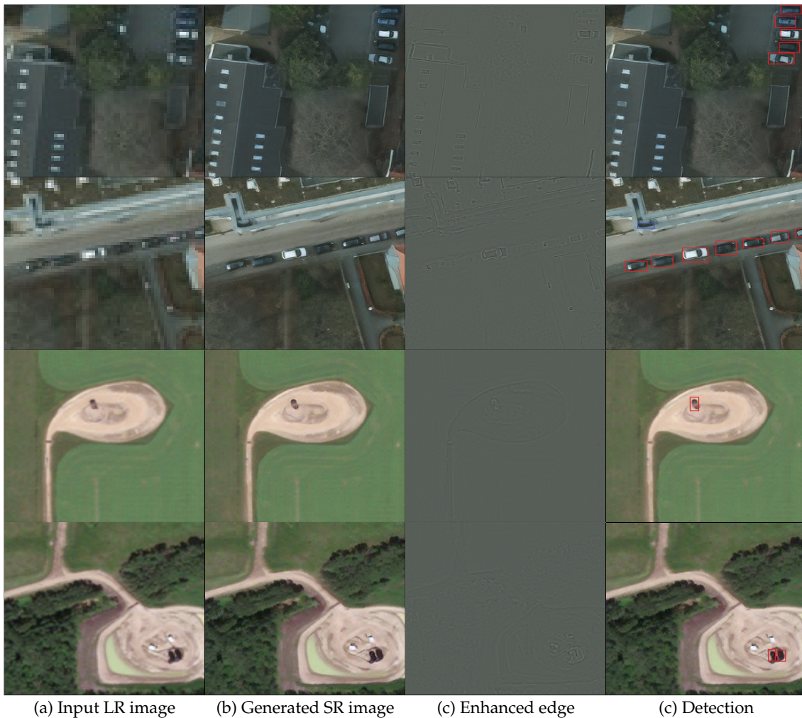
Figure 12. Examples of super-resolution (SR) images that are generated from input low-resolution (LR) images are shown in (a) and (b). The enhanced edge and detection results are shown in (c) and (d). Red rectangles are true positive and blue rectangles are false positive.
