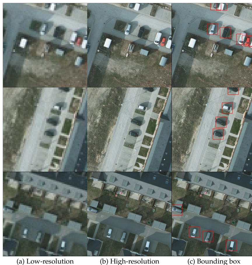
Figure 7. COWC dataset: low/high-resolution image pairs are shown in (a) and (b) and ground truth bounding boxes for cars are in (c).
