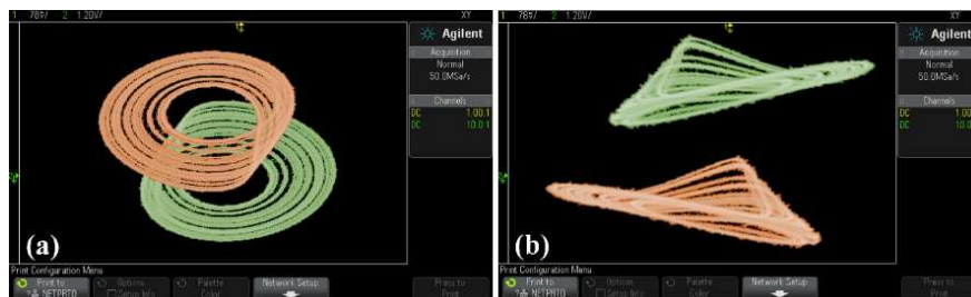
Figure 28. Conditional symmetric chaotic attractors of system (19) with a = 0.6 , b = 1 , c = 2 observed in oscilloscope, (a) z - y , (b) z - x . (IC = (2, 0, -1) is green, IC = (-2, 0, 1) is brown.)
