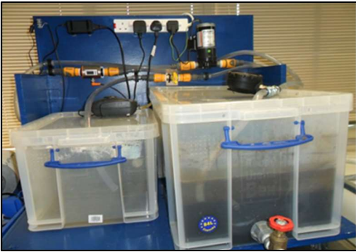
Figure 2. Static square-shaped membrane bioreactor (MBR) system in operation in the laboratory. The square membrane module is located in the larger tank on the right for filtration purposes.
