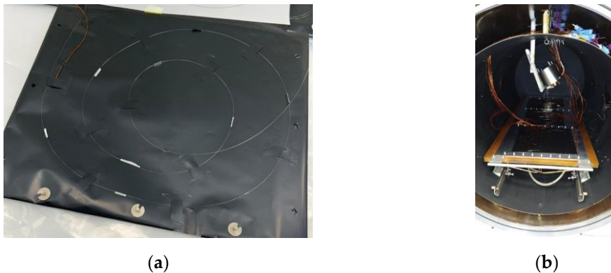
Figure 7 FBG positioning on Kapton support (a) and experimental set-up in vacuum (b).
