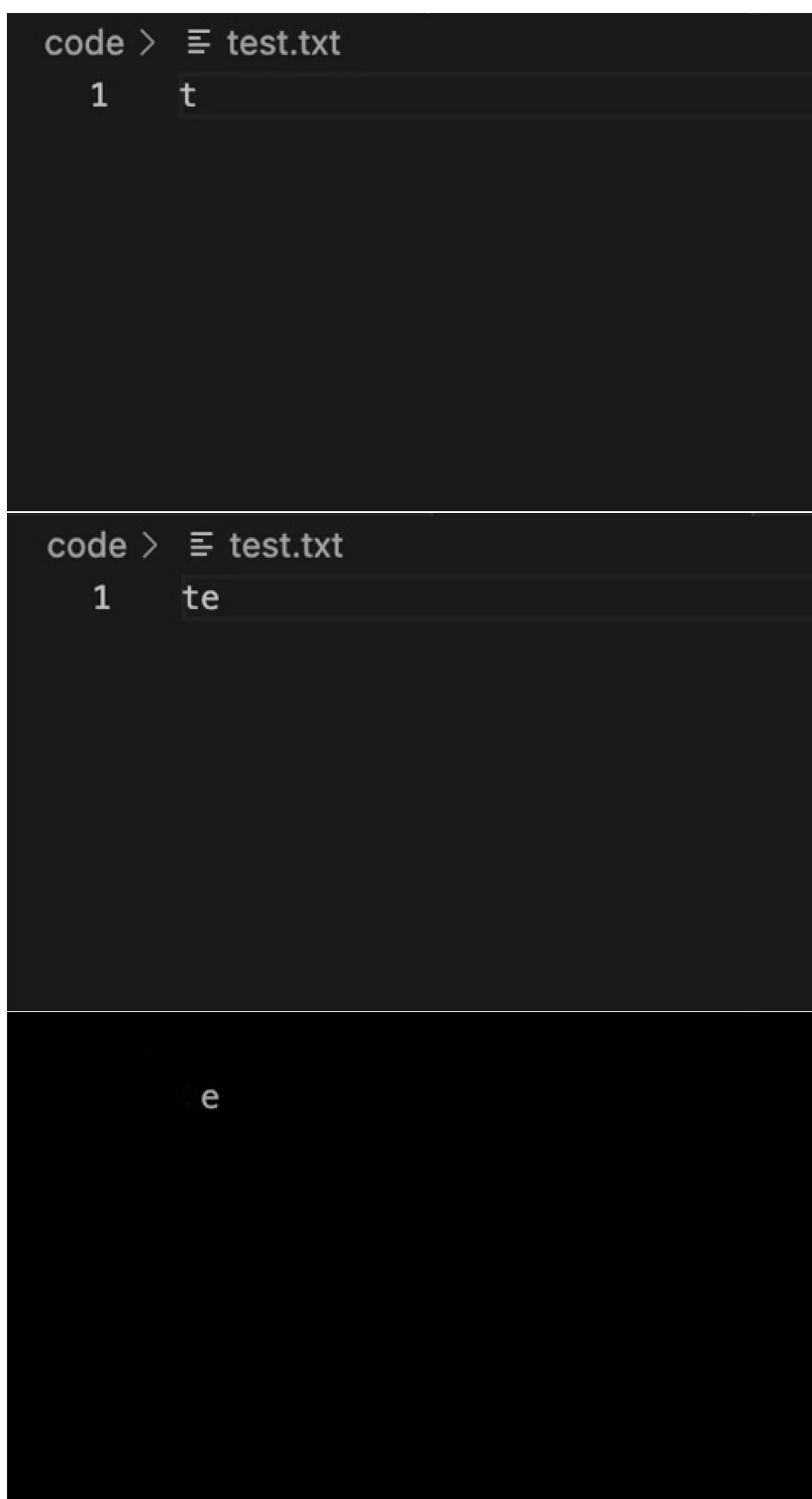
Figure 9. Frames before (left) and after (centre) a key press and their difference (right). The difference image highlights the newly typed character, enabling precise alignment between audio clicks and on-screen input.
