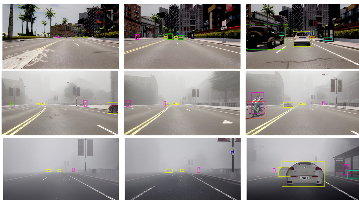
Figure 5. Foggy weather object detection results for the DeepSort-based object detection model. Row 1 is clear weather. Row 2 is medium fog level. Row 3 is heavy fog level [15].
