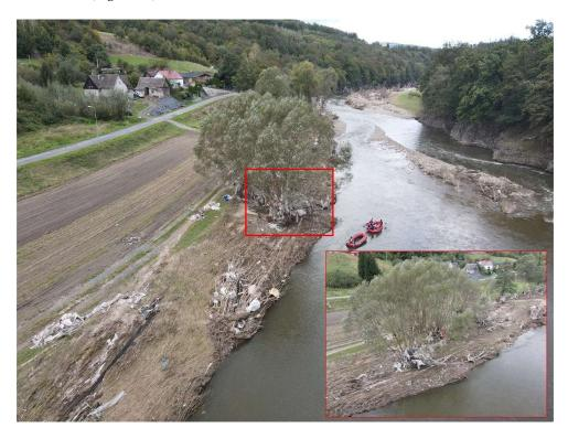
**Figure 19.** Macroplastics accumulated on trees along the Nysa Kłodzka River (123 km) after the September 2024 flood.
