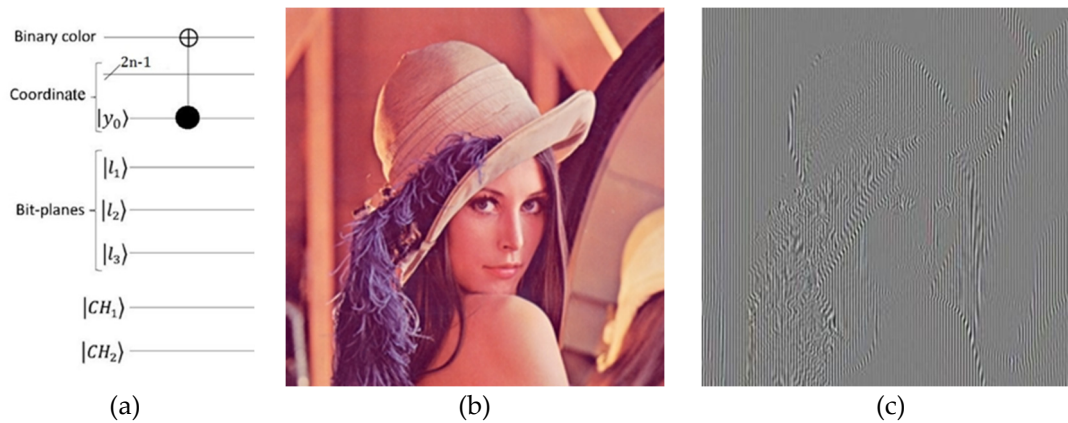
Figure 11. The functioning of color inversion. (a) The execution circuit of U_{XCEP} . (b) A 256x256 image with colors. (c) The outcome of the color inversion process.
