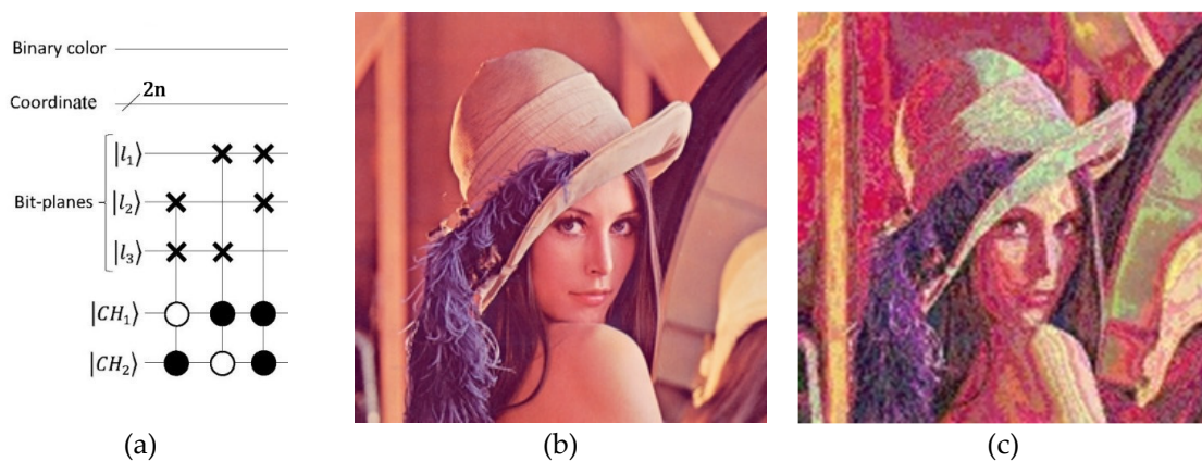
Figure 8. The process of swapping bit-planes involves the following components: (a) The implementation circuit of U_S , (b) a 256×256 color image, and (c) the outcome of the bit-planes swap operation.
