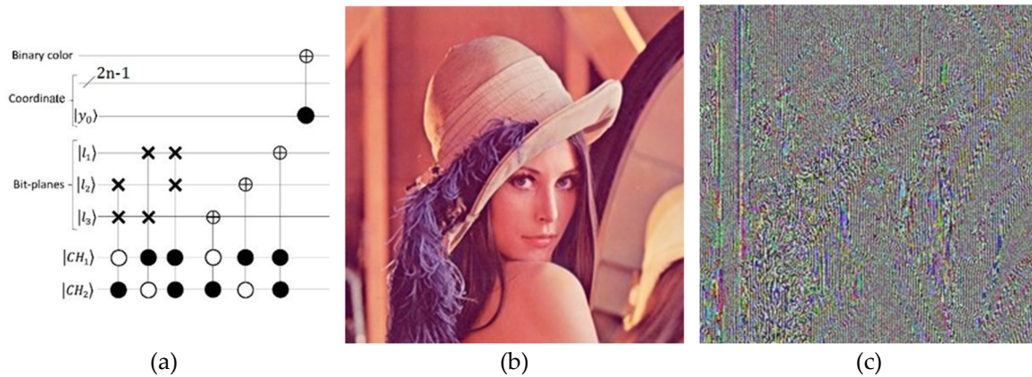
Figure 12. illustrates an image scrambling algorithm that operates on bitplanes. The diagram (a) showcases the implementation circuit of the image scrambling process. In addition, the Lena image is presented in diagram (b). Lastly, diagram (c) demonstrates the encryption of Lena's image through the utilization of the initial phase algorithm.
