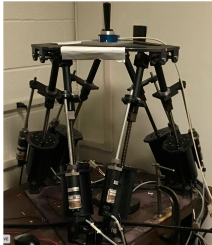
Figure 3. The 6 DOF CKCM manipulator.
