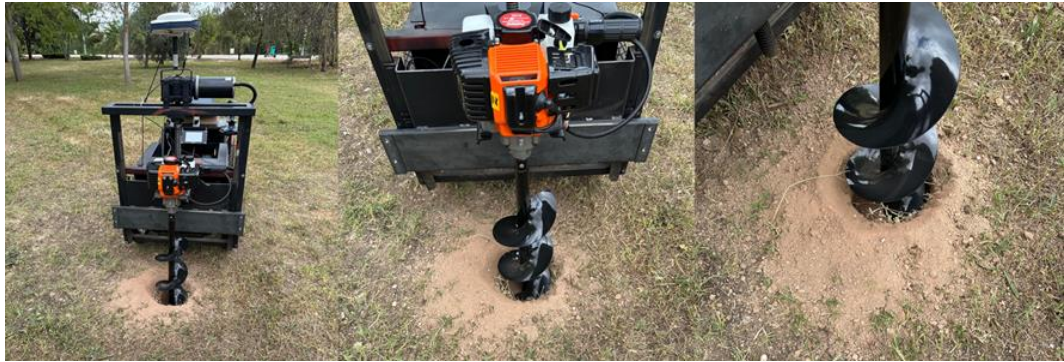
Figure 12. The mobile robot's images in the study field for drilling holes operation.
