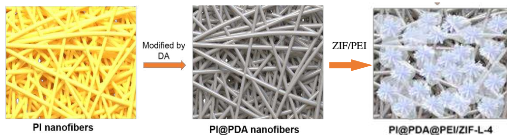
Figure 1. Schematic diagram of preparation of PI@PDA@PEI/ZIF-L composite membrane.
