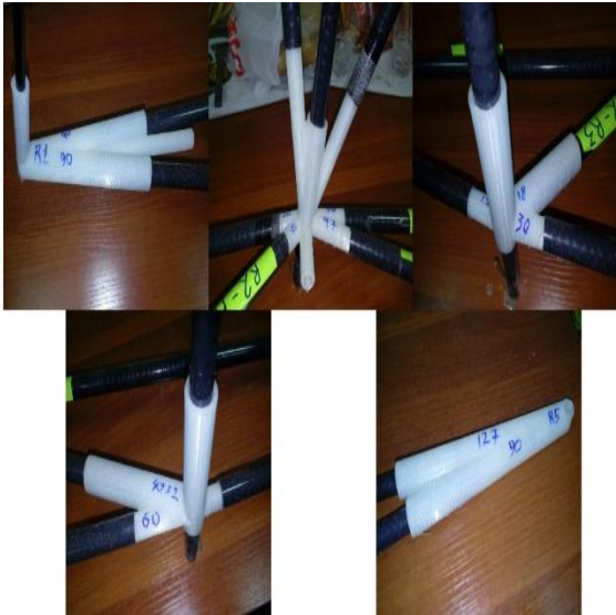
Figure 15. Laboratory testing of epoxy injected assembly joints.
