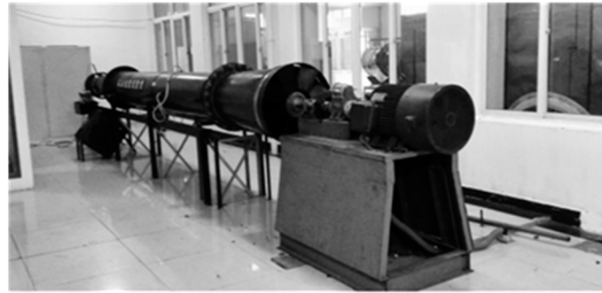
Figure.4. The photograph of fan aerodynamic performance test bench
