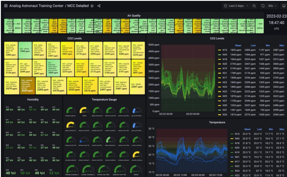
Figure 2. An open source version of Grafana software is used to integrate the sensor data with an internal reporting and monitoring system and to visualize the data.
