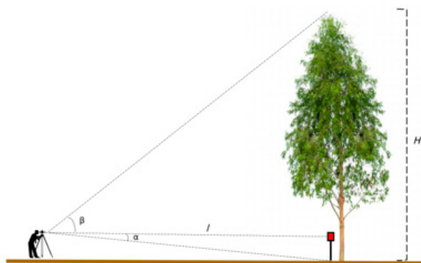
Figure 2. Schematic representation of how the total station was used to measure the total height of E. grandis trees in the field.
