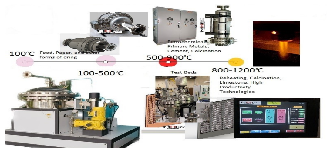
Figure 1. The gamut of heating process temperatures from 100°C to 1200°C with typical use by the industrial sector. (Picture provided by MHI Inc., Cincinnati, USA, reproduced with permission). From left to right, the pictures show electrical steam generation, electrical process gas heating, logic control displays, and the EION system discussed in Section 4.
