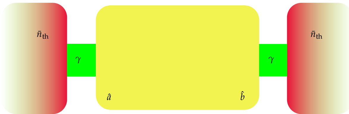
Figure 1. Schematic representation of two bosonic fields, \hat{a} and \hat{b} , both coupled to the same thermal reservoir with average thermal photon number \bar{n}_{\text{th}} . The fields experience decay at the same rate, denoted by \gamma , reflecting identical dissipation mechanisms for each field.
