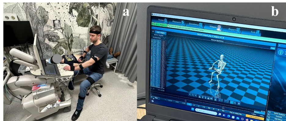
Figure 1. Kinematic evaluation during the testing phase: (a) motion sensors attached to the sonographer’s body, (b) software visualization of motion analysis in real-time.
