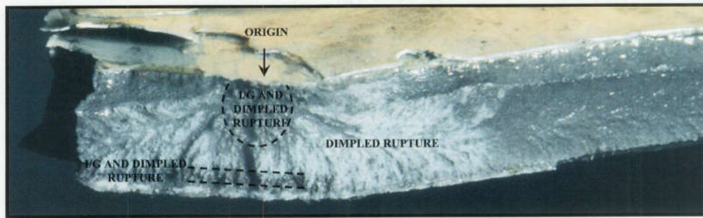
Figure 18. The fracture surface of the CLG cylinder shows the location of the crack and the progression of failure.
