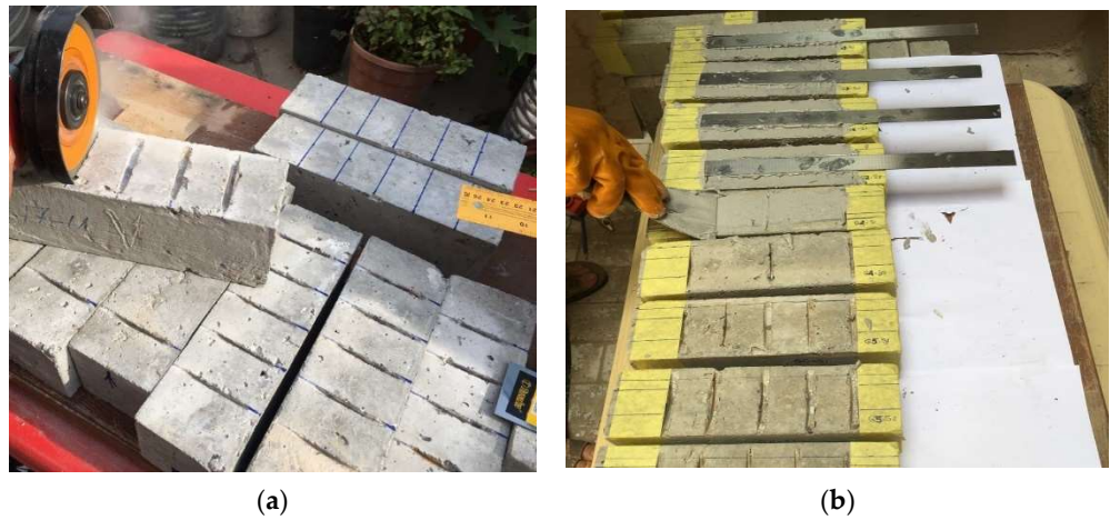
Figure 1. Specimens preparation: (a) Cutting grooves; (b) Application of adhesive.
