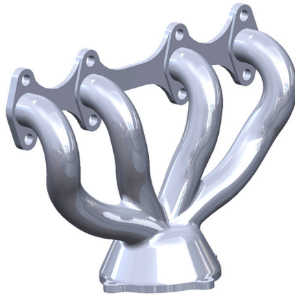
Figure 1. 3D model designed for the modified geometry of the M3 engine exhaust manifold.
