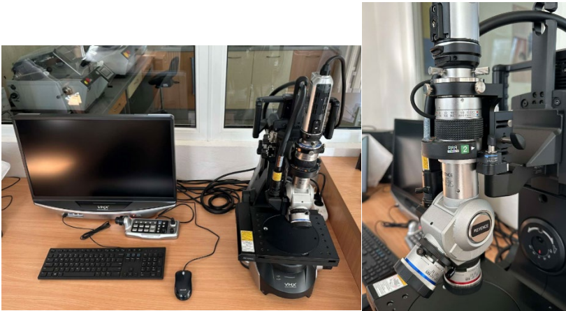
Figure 10. Digital 3D microscope used for angular positioning and evaluation of the cutting blade wear.
