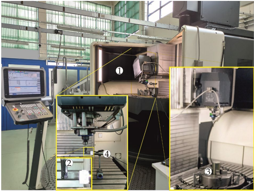
Figure 8. Experimental test bench (1. Machining tool, 2. Torus milling cutter, 3. Workpiece, 4. Dino-Lite 7000 CE series digital workshop microscope).
