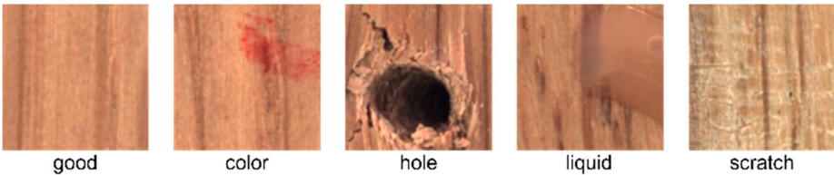
Figure 3. Types of good and defective wood grain patterns.
