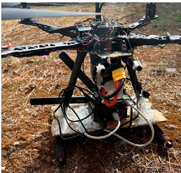
Figure 2. Experimental UAV setup with onboarded connectivity and processing modules.
