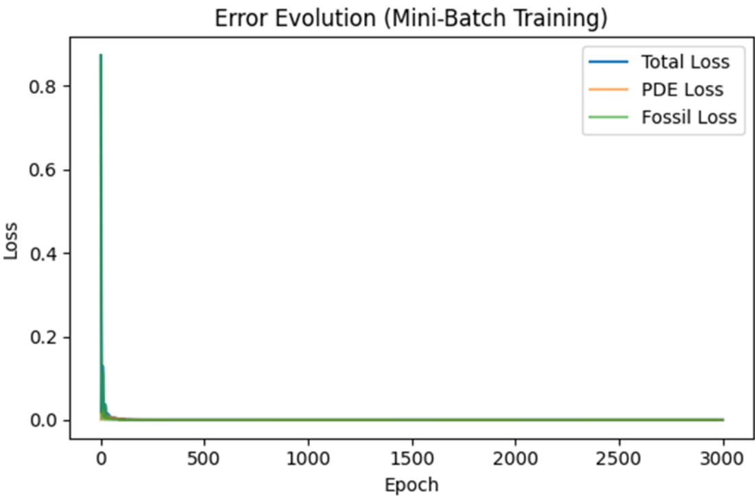
Graph 1. Error Evolution (Mini-Batch Training). A line chart showing Total Loss, PDE Loss, and Fossil Loss as training epochs progress. Early in training, errors are high as the network tries to satisfy both PDE residuals and fossil constraints. Very quickly, losses converge near zero, indicating that the PINN has found PDE parameters and network weights that closely match the fossil data while satisfying the reaction-diffusion equation.
