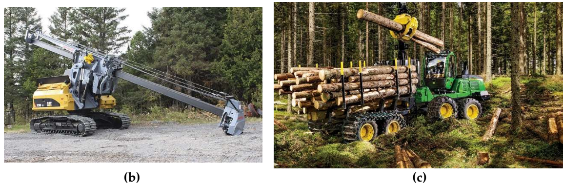
Figure 11. A (a) grapple saw (Cranab), (b) delimber (Pro Pac Industries) and (c) forwarder (John Deere).
