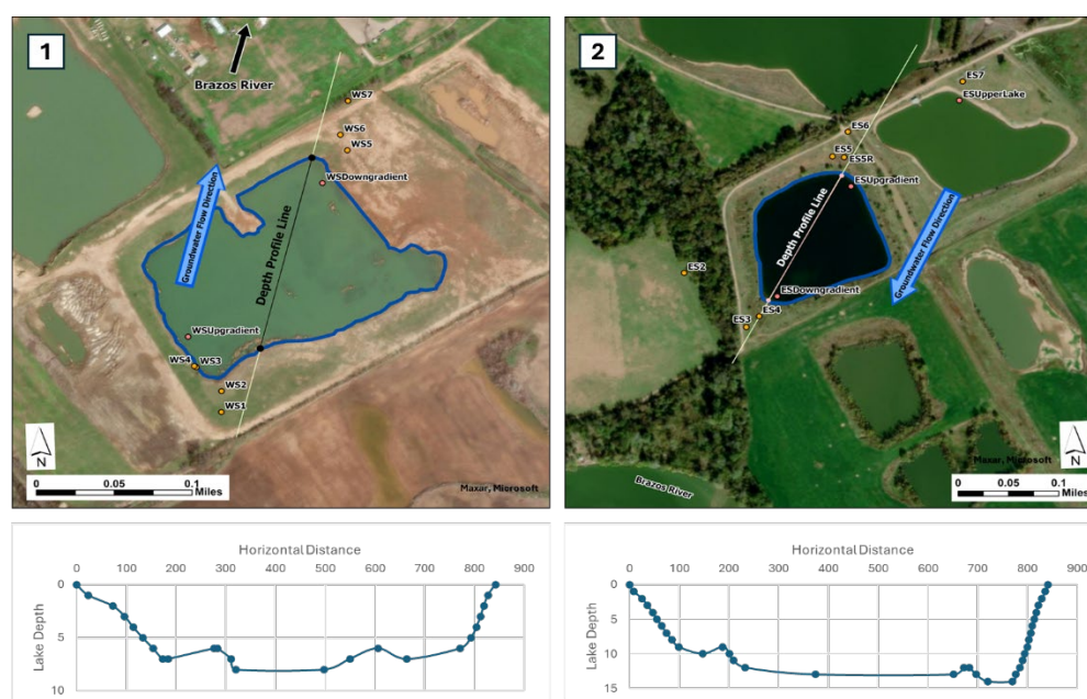
Figure 2. Aerial maps and depth profiles of West Site (1) and East Site (2) Gravel Pit Lakes. Depth profiles were created in the groundwater flow direction for each site. For the West Site this means that the profile is from the southwest to the northeast and for the East Site this means that the profile is from the northeast to the southwest. The white line in each map represents the transect along which figures 9 and 10 were created.
