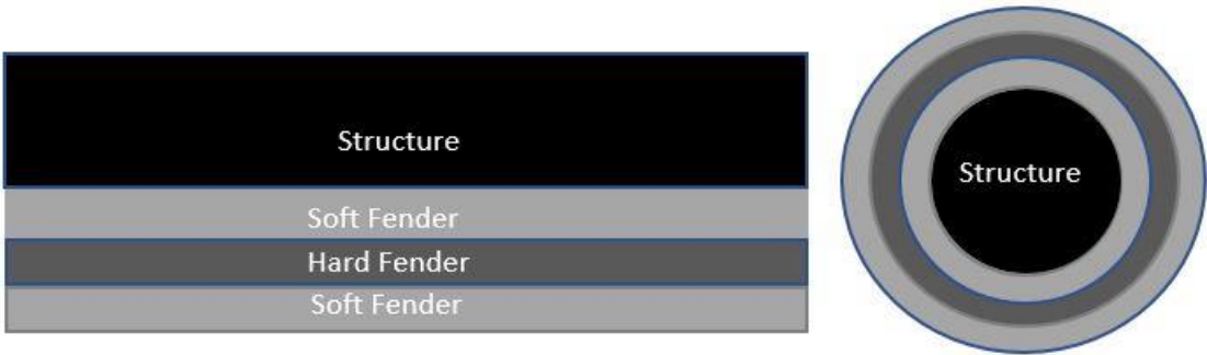
Figure 2. Shows Soft-Hard-Soft Fender design for both Straight and Circular Structure.
