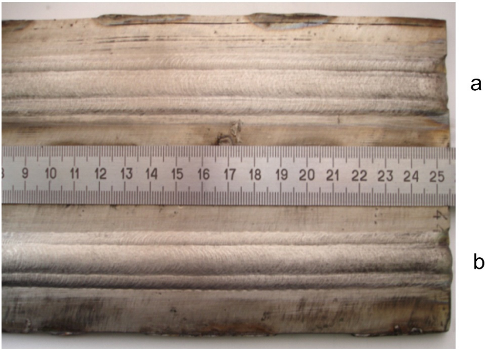
Figure 1. The surface of the sample after the multipass welding seams, made TIG welding in an atmosphere of purified argon: a - wire Filler Metal INCONEL® 52 alloy; b - wire Filler Metal INCONEL® 52MSS alloy.
