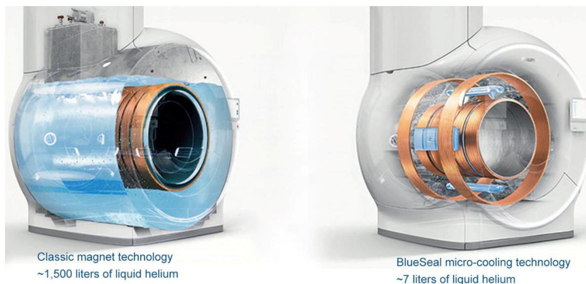
Figure 1. A MRI magnet consists of several coils, each serving a different purpose. The coil that generate the main magnetic field ( B_0 - Principal magnet windings plus superconducting shim and shield coils) is in the center, surrounded by shim coils that help improve the magnetic field homogeneity, not shown are the gradient coils (from here on not in a Helium bath and not superconductive) that are used for imaging (including their active shields), the Radiofrequency (RF) Body Coil (transmits the so called B_1 field), and finally the Patient coils that are used to detect the MR signal (could also be transmit and receive coils). Image courtesy PHILIPS Healthcare (Blue Seal magnet with 7L Helium on the right).
