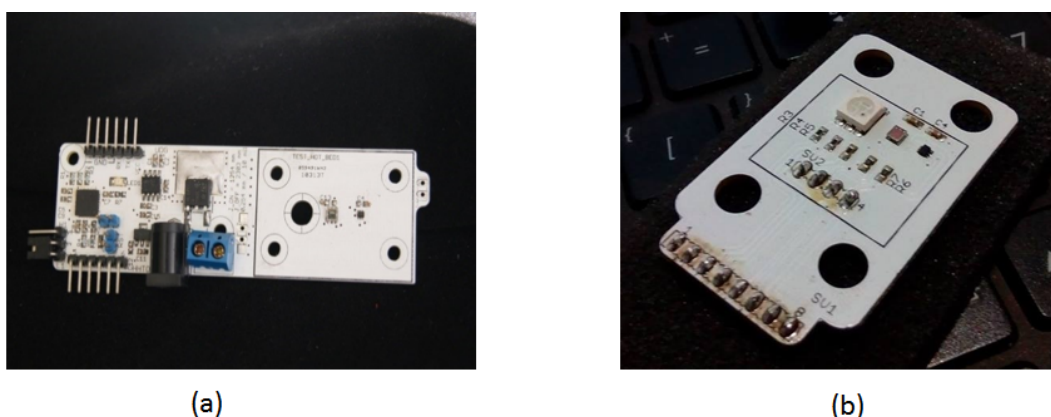
Figure 10. A photo of the assembled control systems for the DNA amplification device. (a) The primary PCB control unit, showing the main components responsible for regulating temperature and system operations. (b) The secondary control PCB with a protective cover, which houses additional circuitry for managing the device's sensor inputs and outputs.
