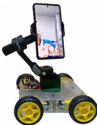
Figure 3. Functional prototype of the constructed Selfie Robot featuring the 4WD platform, three SG90 servo arm, and integrated electronics (Arduino Nano, HC-05, L298N, Li-Ion battery).
