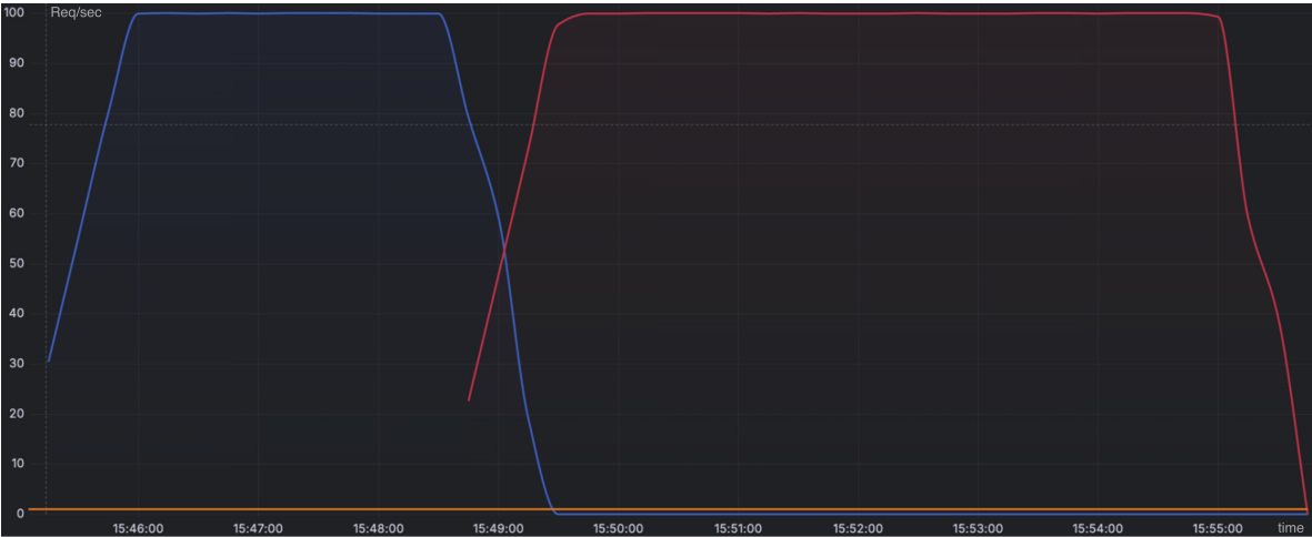
Figure 6. Traffic shift during Kubernetes deployment change Legend: — Deployment availability, — Successful requests, — Failed requests.
