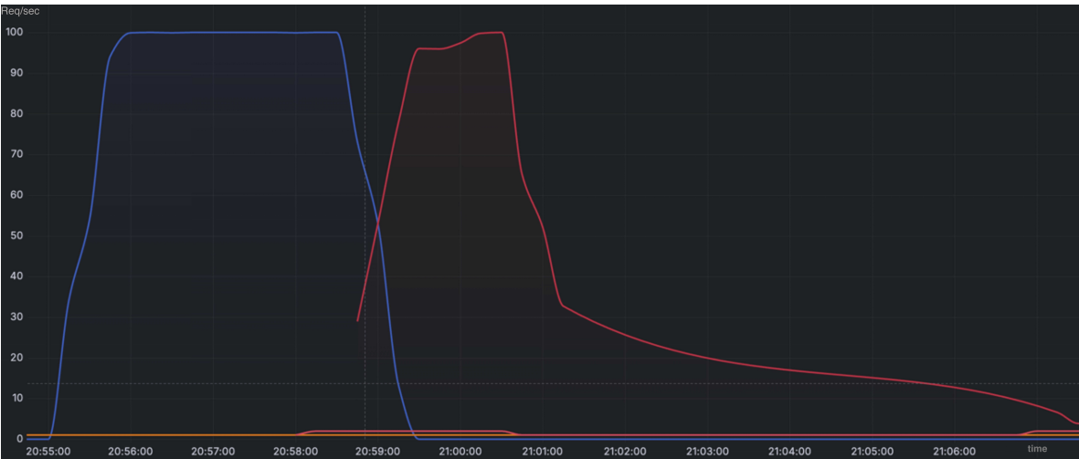
Figure 8. Traffic shift during Kubernetes deployment change Legend: — Blue deployment availability, — Successful requests by the blue deployment, — Failed requests by the green deployment, — Green deployment availability.
