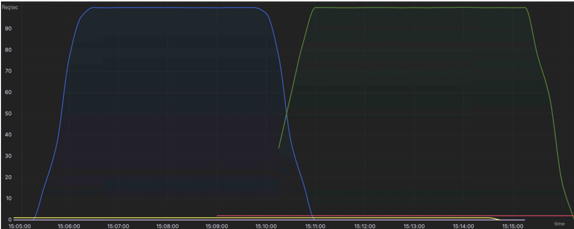
Figure 12. Traffic shift during kubernetes deployment change Legend: — Blue deployment availability, — Successful requests, — Green deployment availability, — Successful requests by the green deployment.
