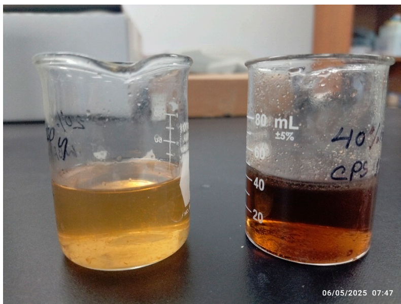
Figure 6. (a) Effect of acid concentration and treatment duration on weight loss, (b) the thicker and slurry solution after 2 days of dissolution (right side), 40% acid solution (left side).
