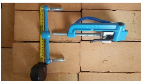
Figure 14. Barbero Mauser strapping system for stainless steel strapping: Model B05.T000S262.
