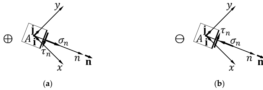
Figure A3. Stress components acting on the plane with unit normal vector \mathbf{n} (the plane perpendicular to the outward-pointing line n ) in the reference frame of Figure A1: (a) For normal and shear stresses that are positive in the Mohr plane; (b) For normal and shear stresses that are negative in the Mohr plane.
