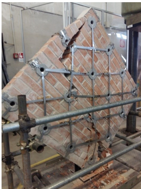
Figure 21. Failure mode of Specimen M2-45.
