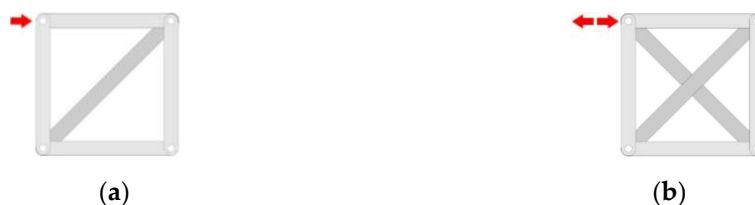
Figure 3. Bracing of a rectangle made of hinged strips: (a) By adding a strip along a diagonal, which will prevent the rectangle from collapsing in one direction but not the other; (b) By adding strips along both diagonals, which will prevent the rectangle from collapsing in either direction.
