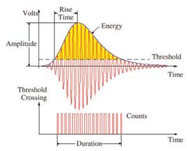
**Figure 2.** The definitions for acoustic-emission parameters [24].
