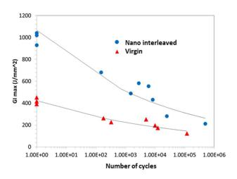
Figure 4. G<sub>Imax</sub>-Na for the fatigue tests calculated based on ASTM D6115 [22].
