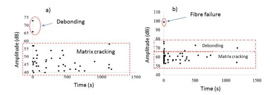
**Figure 7.** AE signals Amplitude distribution versus time for the fatigued samples (a) Virgin and (b) Nano-interleaved.
