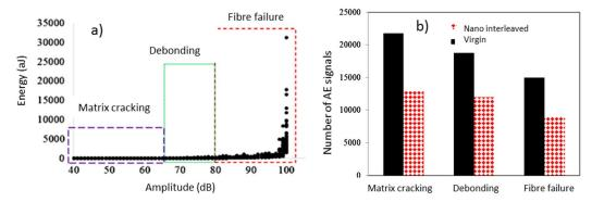
**Figure 6.** (a) Classification of the AE signals based on their Energy and Amplitude levels, (b) Number of AE signals associated with different failure mechanisms for the static loading.
