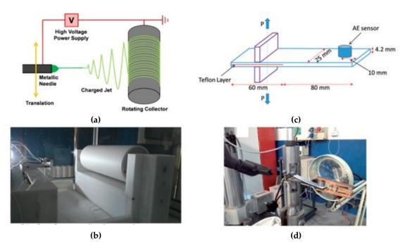
**Figure 1:** Electrospinning and testing equipment: (a) Schematic of the electrospinning process. (b) The electrospinning equipment. (c) Schematic of the DCB specimens. (d) DCB specimens and experimental setup.
