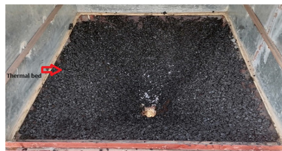
Figure 2. Thermal bed (Basalt-biochar) inside the solar dryer.
