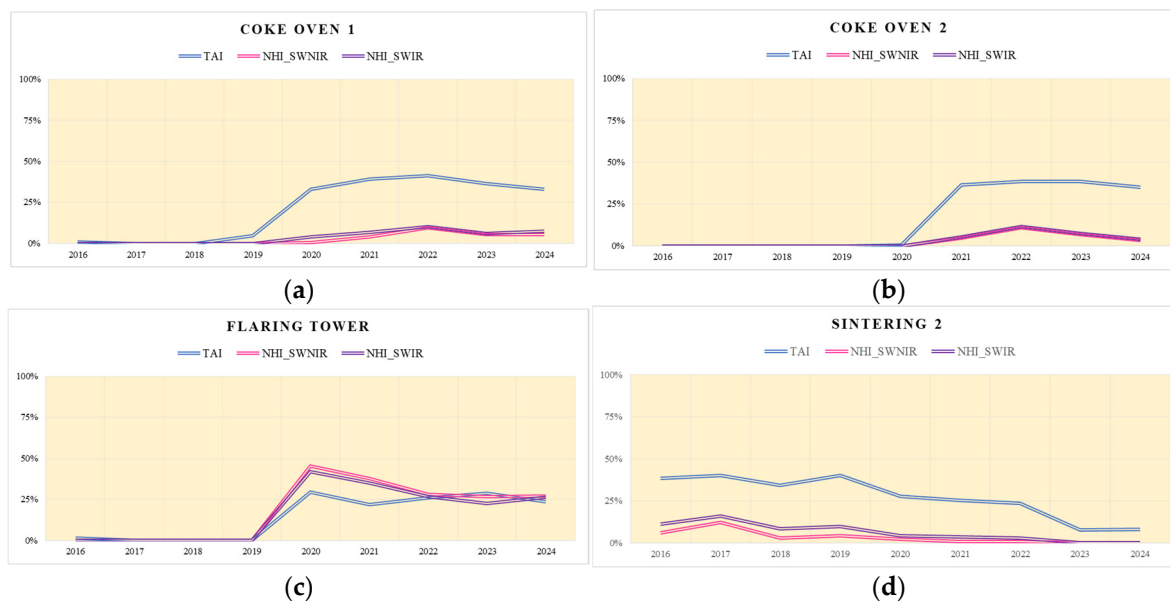
Figure 10. Annual percentage of activations recorded for Gijón sub-assets (a) coke oven 1; (b) coke oven 2; (c) flaring tower and (d) sintering 2. Activations are shown for TAI (blue line) and NHIs (pink line for NHI swnir , purple line for NHI swir ) over the period 2016-2024. The table in the top-left corner quantifies the percentage of activations by metric type.
